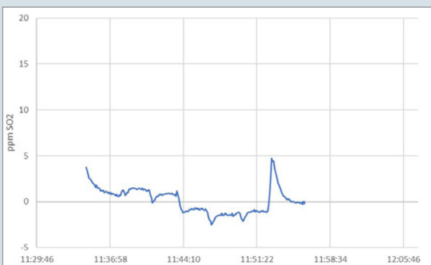
Fig. 5a/b: Response of a CO-insensitive SO 2 sensor TSCi to SO 2 and CO (uncompensated)
